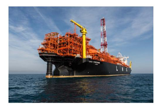
**OLT Offshore LNG Toscana Spa** developed and implemented the regasification Terminal "FSRU TOSCANA". OLT is the owner and the manager of the Terminal. The Terminal is located at 22 km offshore the Tuscan coast and it is connected to mainland by a 30 Km approximately of pipeline which is used to send natural gas to the Italian national grid.
