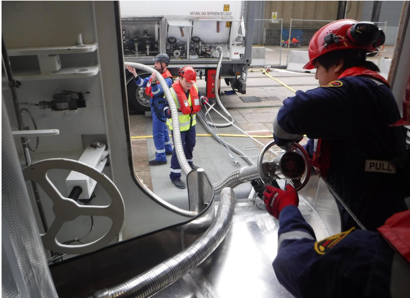
HANDLING OF TRANSFER HOSE
