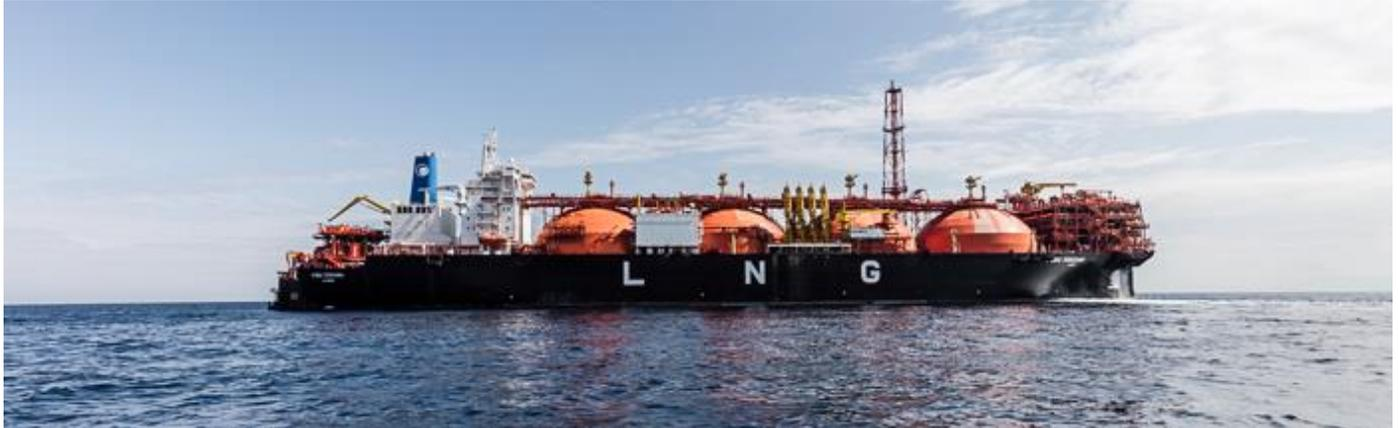
**OLT Offshore LNG Toscana S.p.A.** is the company that developed and now owns and manages the floating regasification Terminal FSRU Toscana. The Terminal is permanently moored about 22 km off the Tuscany coast between Livorno and Pisa and it is connected to the mainland through a subsea pipeline, through which natural gas is sent to the Italian national distribution network.
